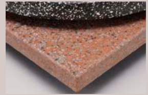
260 1/4" Eased Flat Edge. 1/8" veneer solid surface material over a 3/4" exterior grade plywood core.
